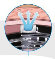
The Abluminal Reservoir Technology allows a sustained drug release, exclusively towards the vessel wall, up to 3 months
